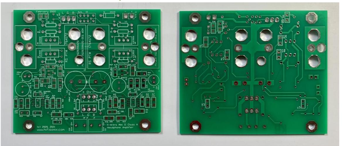
The large holes in the PCB allow airflow up through the vertically mounted heatsinks. The temperature rise above ambient for 45mm high heatsinks is about 8 C (Image updated 15 May 2023)
