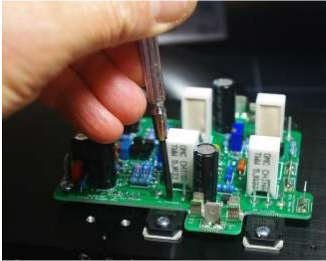
Figure 19 - Apply pressure to PCB when soldering
