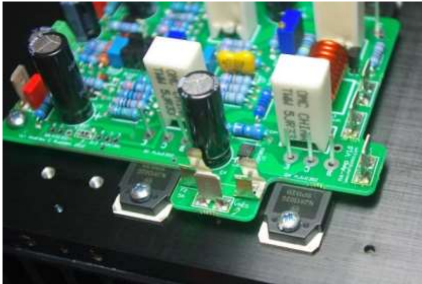
Figure 16 - PCB + Heatsink assembly prior to soldering the power devices. In photo, it is the nx-Amplifier board that is shown – the sx-Amplifier assembly is exactly the same
