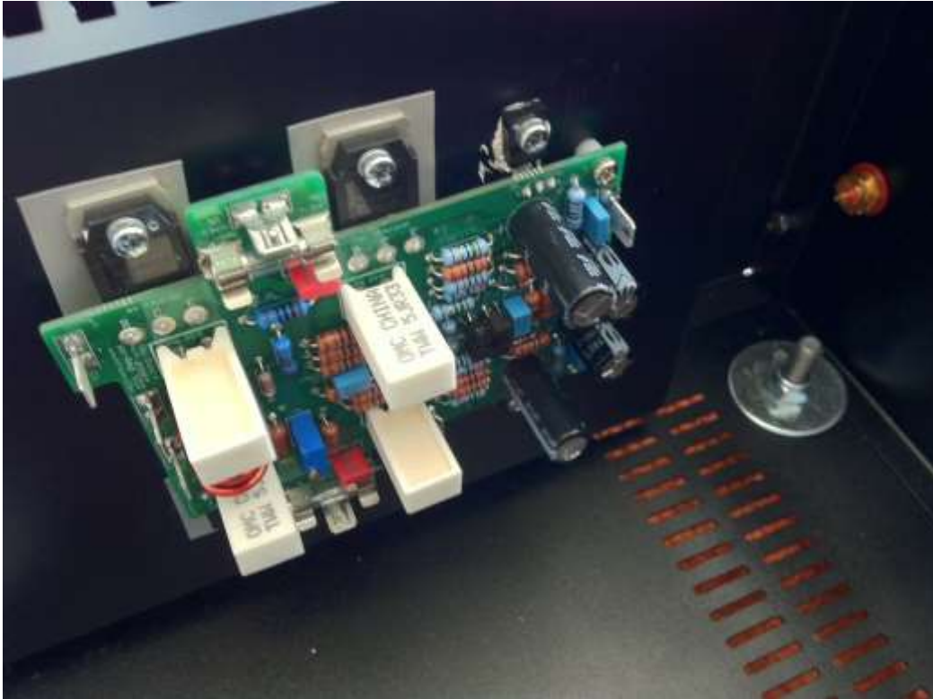
Photo 5 - A view of the Amplifier Module on the Heatsink Prior to Wiring
