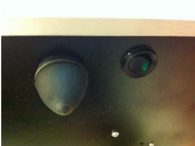
Photo 7 - Amplifier Housing Feet - Large Rubber Bumpers Ensure Good Airflow Under the Chassis
